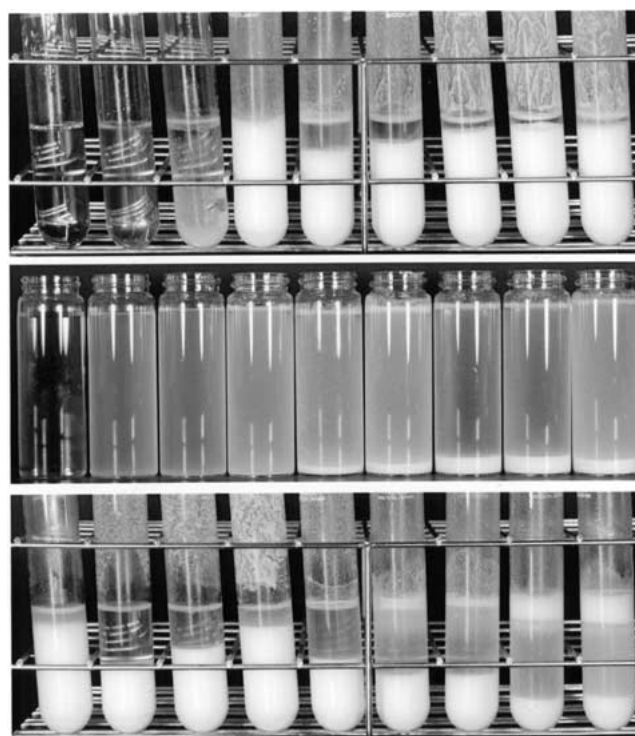
Figure 3. Photograph of inclusion complexes with unsaturated aldehydes. Upper, α-CD; middle, β-CD; lower, γ-CD. Aldehydes were left to right as follows; crotonaldehyde, trans -2-pentenal, trans -2-hexenal, trans -2-octenal, trans -2-heptenal, trans -2-octenal, trans -2-nonenal, trans -2-decenal, trans -2-undecenal and trans -2-dodecenal.
